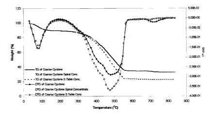
Fig. 3. TG and DTG curves of coarse cyclone circuit underflow and coarse cyclone circuit underflow concentrate by humphreys spiral and shaking table
